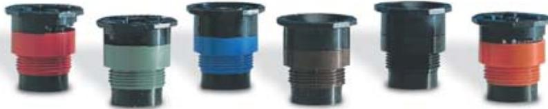
Matched precipitation rate nozzles apply water at approximately the same rate. Preinstalled PCD's eliminate fogging, conserve water and provide precise flow rates. Complete selection of spray patterns and trajectories add to versatility with flow rates from 0.05 - 4.58 GPM (0,2 - 17 LPM).
