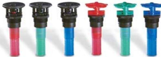
Pre-assembled nozzle, adapter and pressure compensating screens are ideal for ground cover, flower beds and low-water use plants. Four nozzle patterns and three radii available with flow rates ranging 10 - 31.6 GPH (40 - 119,6 LPH).
