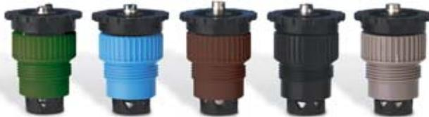
Balanced precipitation rates within TVAN families fit all Toro 570Z sprinkler bodies. Adjustable from 0 - 360° with five different color codes for easy radii identification (8' - 17').
