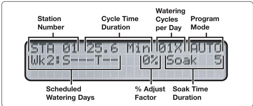
In the example above, Station 01 cycle time is 25.6 minutes, one time per day and is assigned to the “Fully Automated” program mode. If the assigned program mode is “User Programmed-With ET Service Active” “U-ET” will be displayed. “U-NO” will be displayed if the “User Programmed -With ET Service Inactive” program mode is used.
