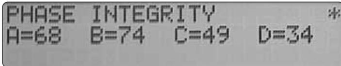
**Note:** If a value of 32 or above is not indicated, install external antenna kit, P/N 102-5581 to increase reception strength.
