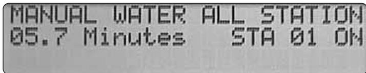
**Note:** Cycle time can be adjusted with the Lower Line dial while the station is operating. Selecting 00 minutes turns off operation.
