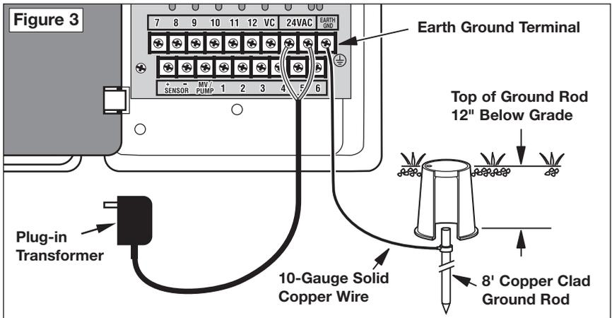
**▲ CAUTION:** The controller’s surge protection circuitry must have an earth ground path to function properly. Proper grounding is especially important in lightning-prone areas.
