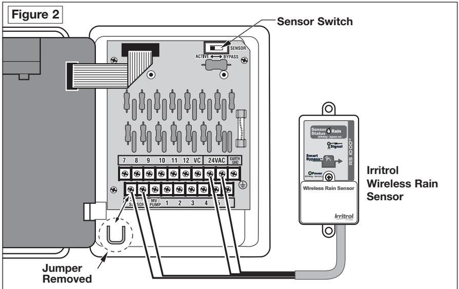
1. Insert in the sensor connection cable through the access hole in the bottom of the cabinet.
